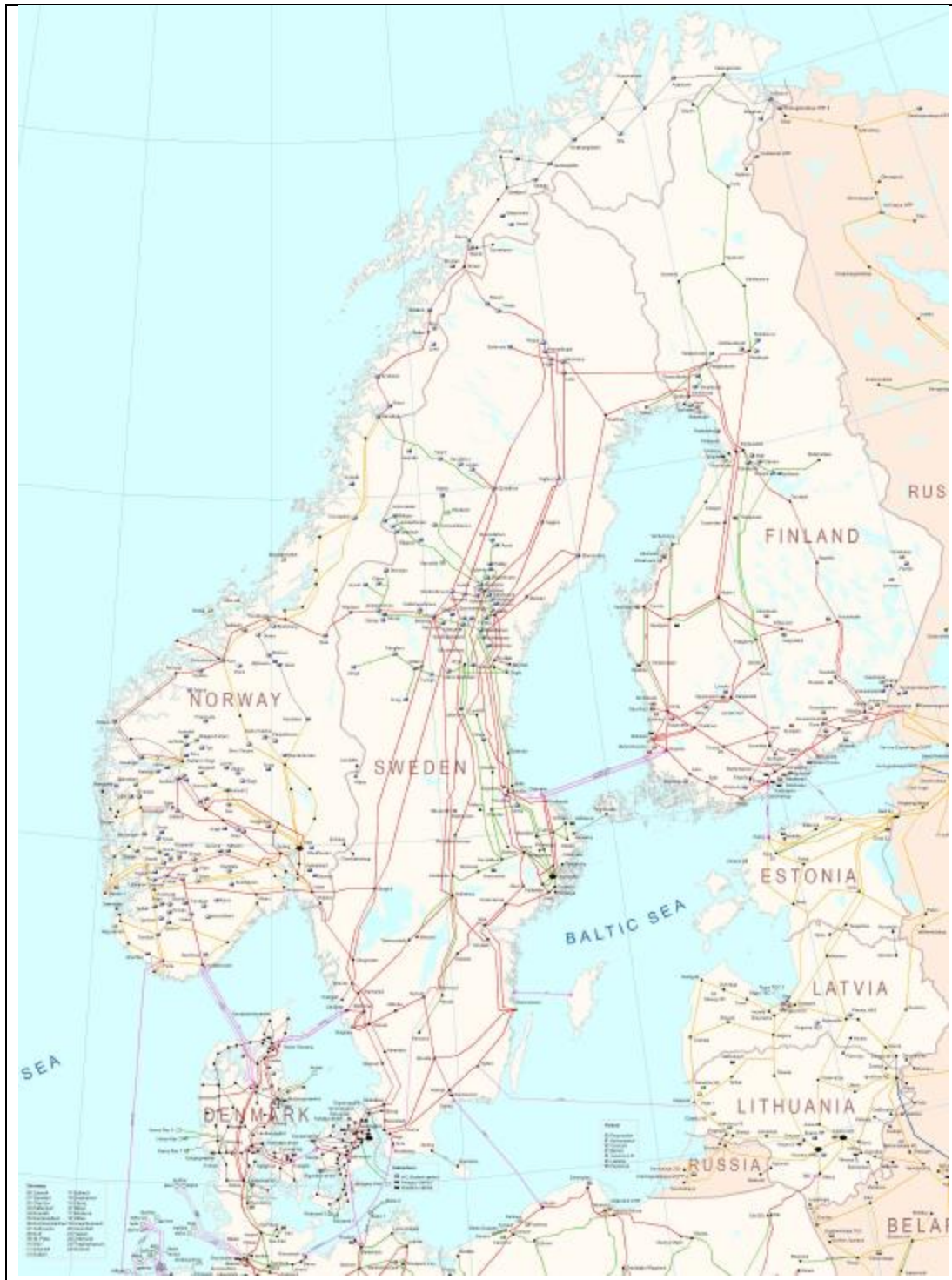
Figure 2 Map showing the Nordic power system (ENTSO-E, 2016). The transmission grid is needed to transport electric power from sites of generation to sites of consumption, but this grid has a limited capacity to transmit electric power.
